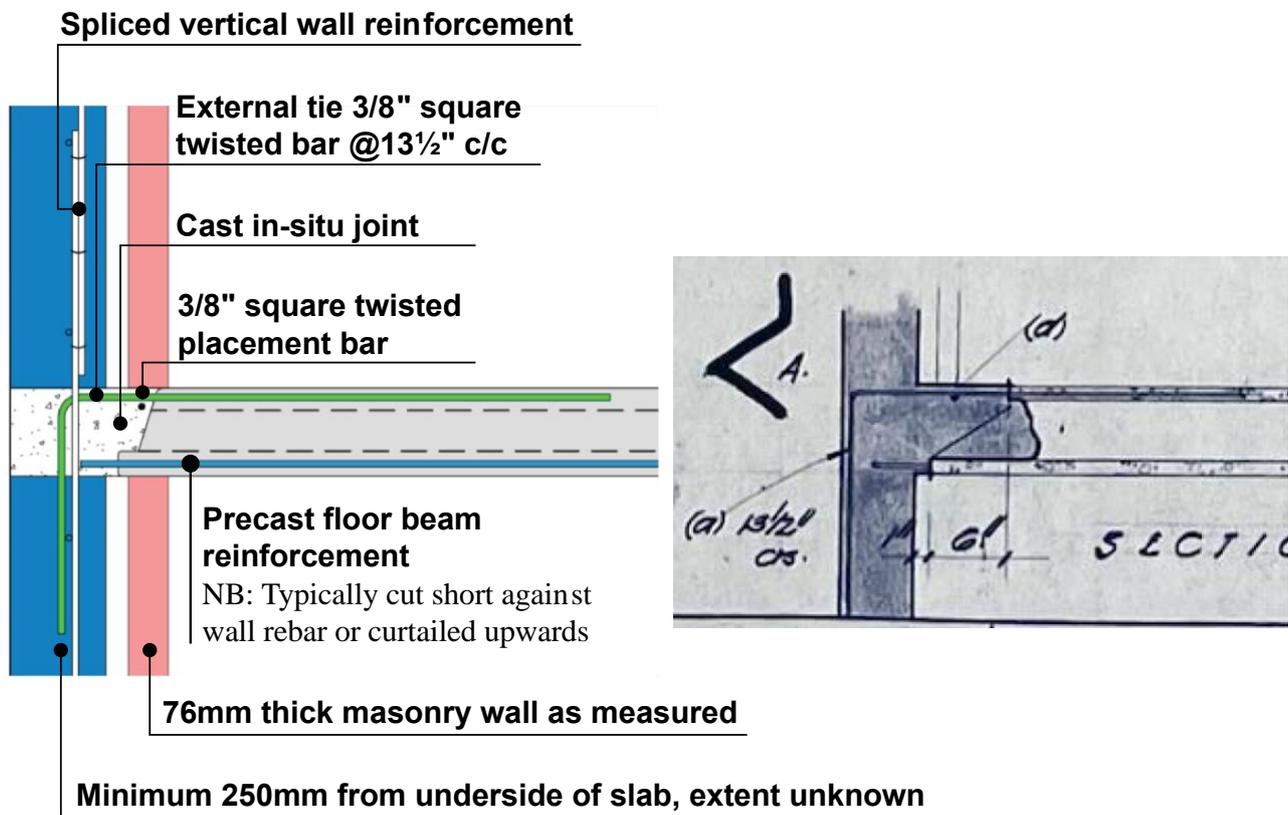
The original drawings specify cover to steel reinforcement above ground to be 1” (~25mm); therefore, it is believed the original intent was to provide ~25mm of cover to the steel reinforcement in flank walls. Typical cover measurements exceeded the 25mm intent in the record drawings. By exception some locations of low cover were observed (as described for internal cross walls); in these instances, a 40mm shotcrete layer was observed on the inner face of the flank wall.
