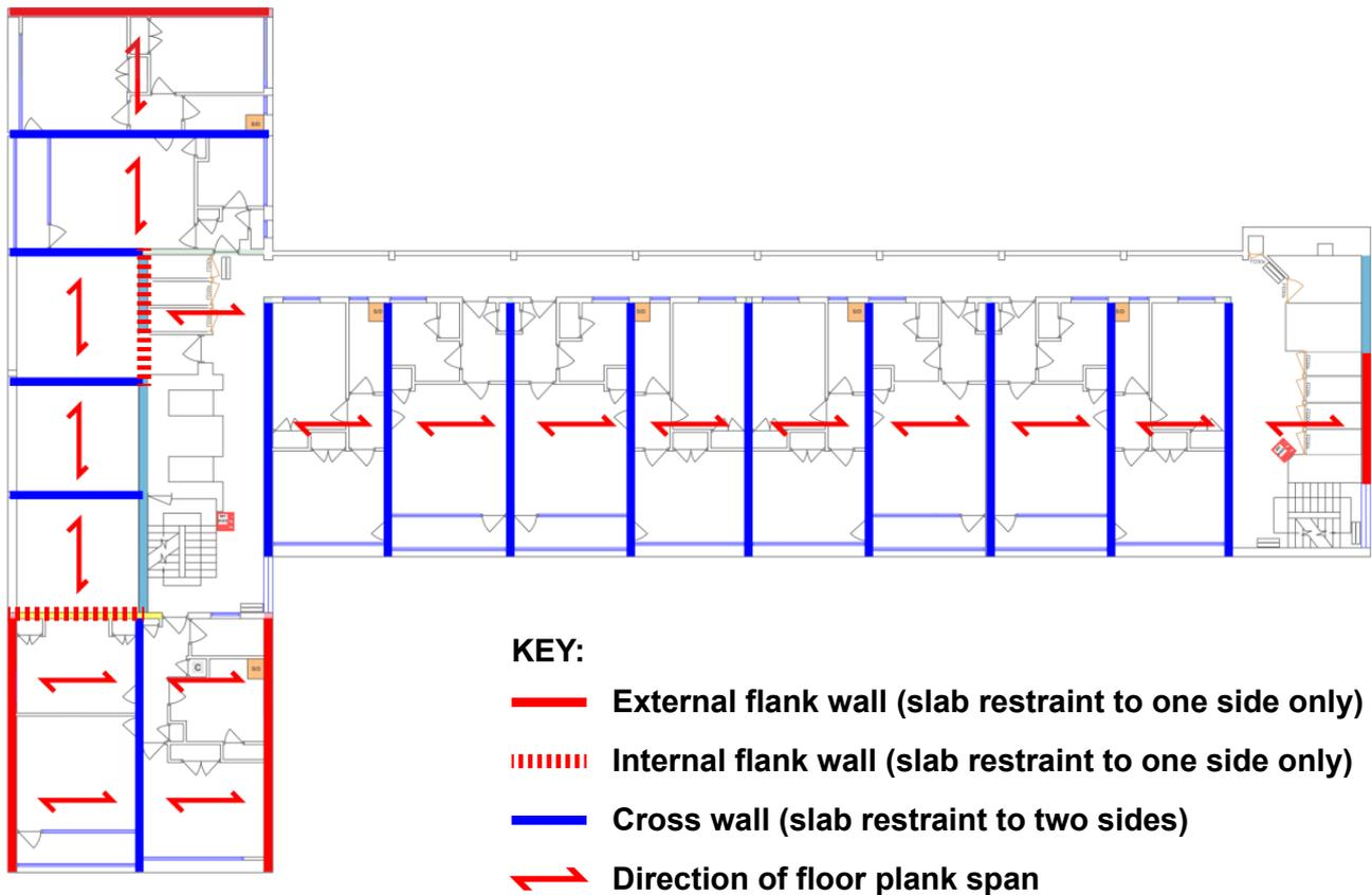
Arup's understanding of the structure of Barton House is built up from a combination of the record drawings and site survey information obtained by Ridge and observed by Arup. The relevant details of the structure, as considered in the structural fire analysis are summarised below.
