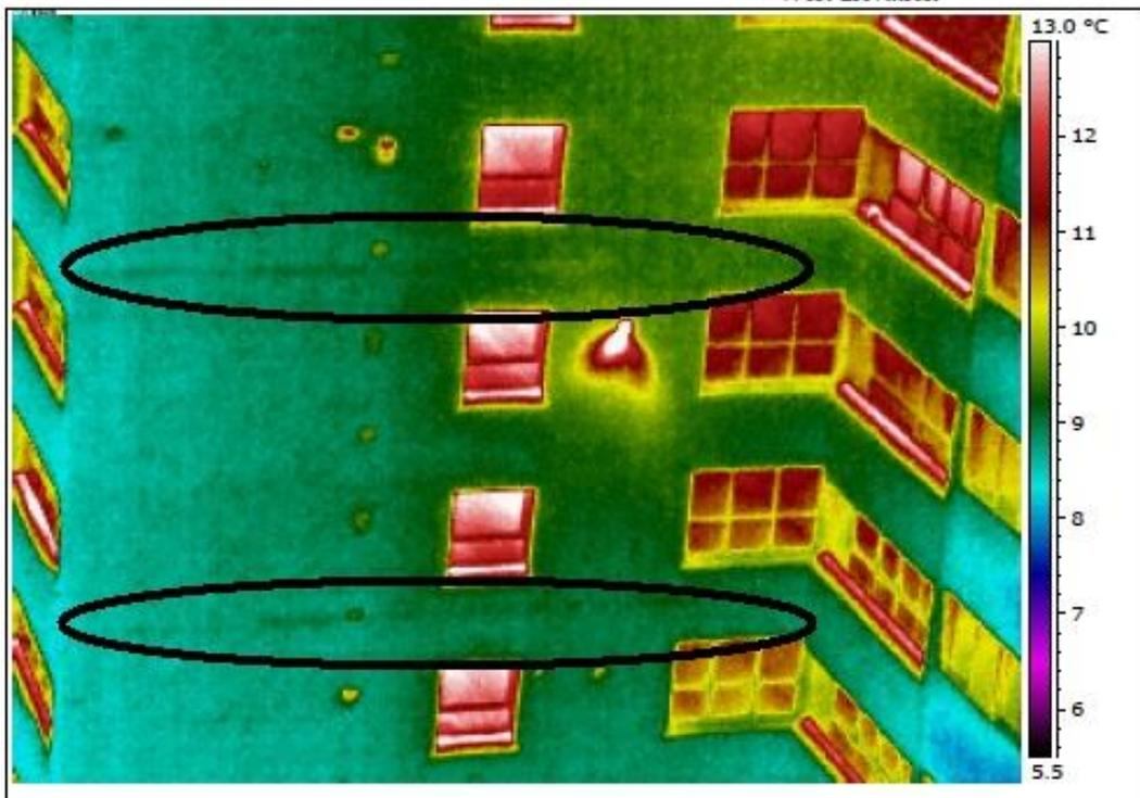
1, 2 and 3. Thermal image of typical elevation 3 showing defined thermal signature for barriers at alternate floor slab levels as confirmed in photo below.
